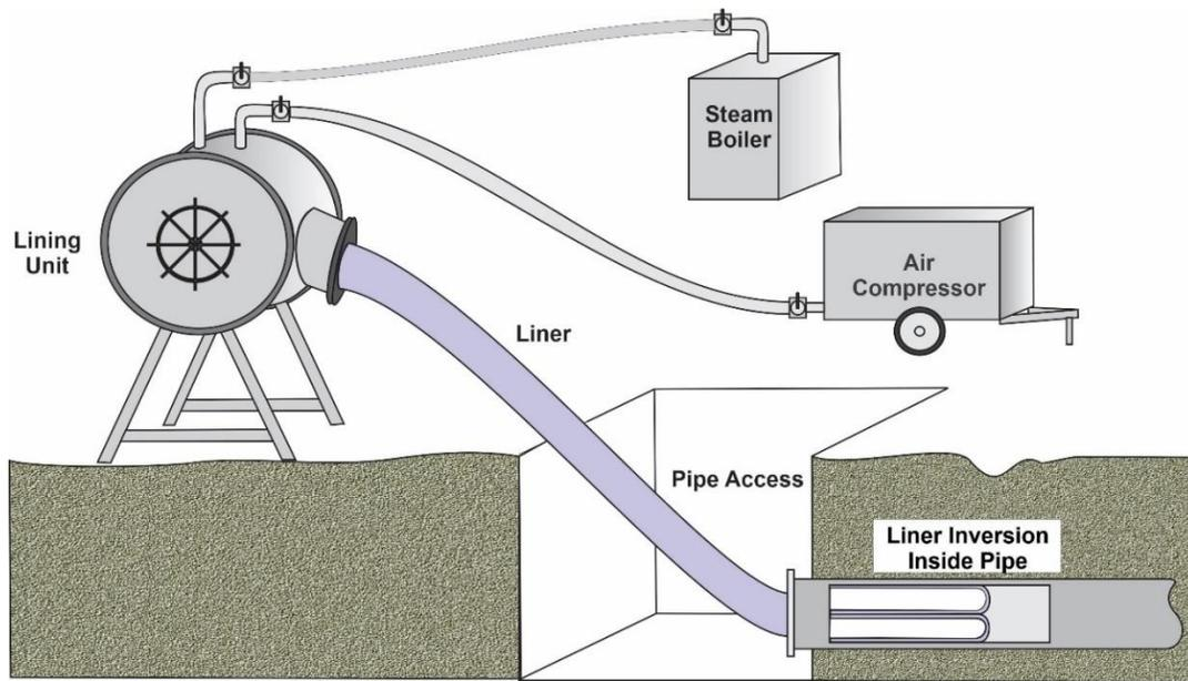
Schematic Drawing of CIPP Installation with Air
