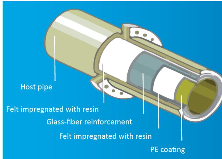
**Figure 1 Schematic of an installed CIPP liner in a pipe [Error! Reference source not found.]**
