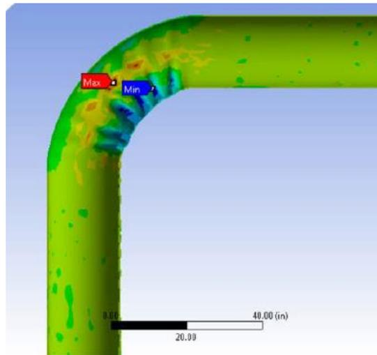
Bending Moment Analysis - Wrinkled CIPP Elbow
