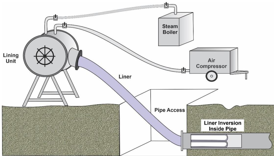
Schematic of CIPP Installation with Air
