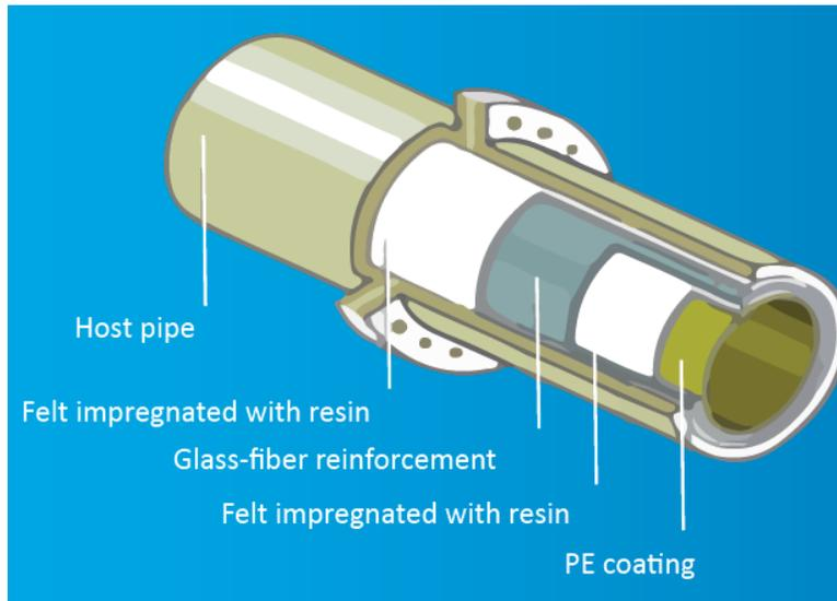
Schematic of an installed CIPP liner in a pipe [5]
