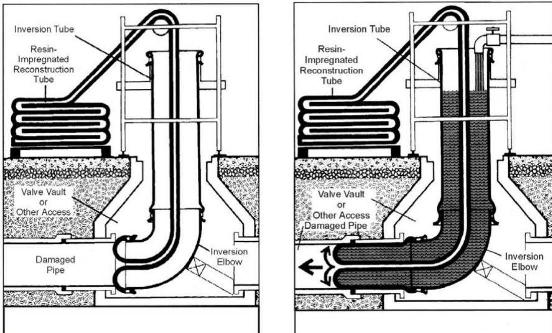
Schematic of CIPP Installation with Water [1]
