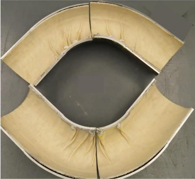
Cut Out of a 90° Elbow (8” NPS) Lined with CIPP
